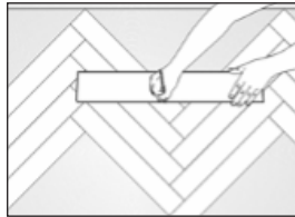
Figure 10: Adjust the starting rows. The first four rows have to be cut parallel to the wall. Measure and mark where to cut the floor panels at a fixed / parallel distance to the wall.
