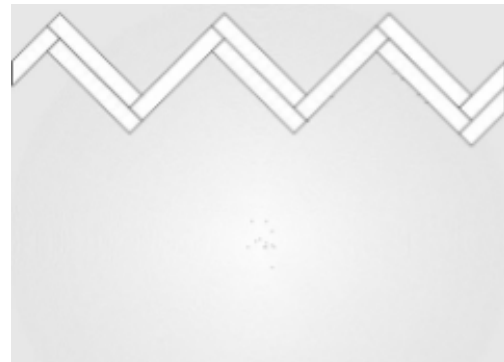
Figure 7: Install the A-panels. Continue from the left to the right and install all the A-panels in the second row. Finish with a piece of panel cut to size (step 5).
