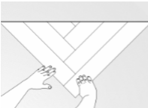
Figure 12: Install the starting triangles. Connect the cut starting panels to form triangular shapes, one by one. Start installing the triangles from the left corner. It is recommended to use glue to fix the smallest parts of the triangles into place by applying a small quantity of glue inside the groove.
