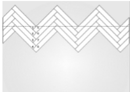
Figure 11: Number the panels from 1 to.... This will allow you to keep the panels in order. Dismantle the panels and cut them to size along the previous marked line.
